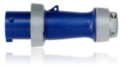
UPC Code : 078477901625 Country Of Origin : Mexico 60 Amp, 250 Volt 3-Phase, 3P, 4W, LEV Series North American-Rated IEC 60309-1 & 60309-2 Pin & Sleeve Plug, Industrial Grade, IP66/IP67/IP68/IP69K, Watertight - Blue
